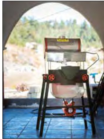
An electric corn grinder waits for power. This machine will take a 5-hour daily task and reduce it to about 10 minutes. Villagers will also be able to store the ground corn in a refrigerator and not have to do this task every day.
